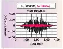
Fig. 5 Time domain of 'system' S<sub>1</sub> with superimposed time domain of desired signal.
